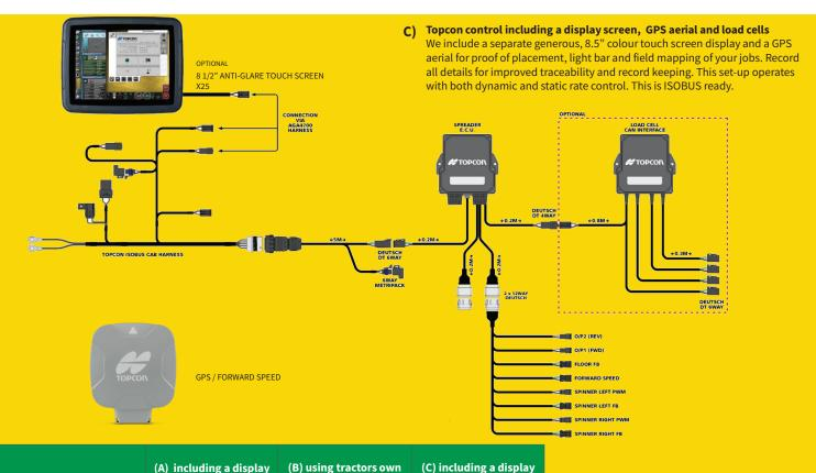
(A) including a display screen and GPS aerial but no load cells (C) including a display screen and GPS aerial with load cells
