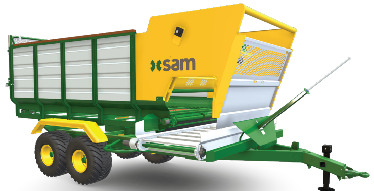
10 cube tandem-axle, chain side-feed Both shown on 400/60 x 15.5 tyres (an upgrade)
